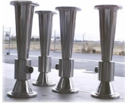
The Outlet Pressure is independent of the Inlet Pressure, which is usually delivered by a pump. For example, if pressurized water is flowing through an Injector and runs down a short pipe and simply falls on the ground, the Outlet Pressure (back-pressure) is nearly zero. Any restrictions downstream in the form of piping, filters, valves, sprinklers, emitters, etc. cause the Outlet Pressure (or back-pressure on the Injector) to change.
