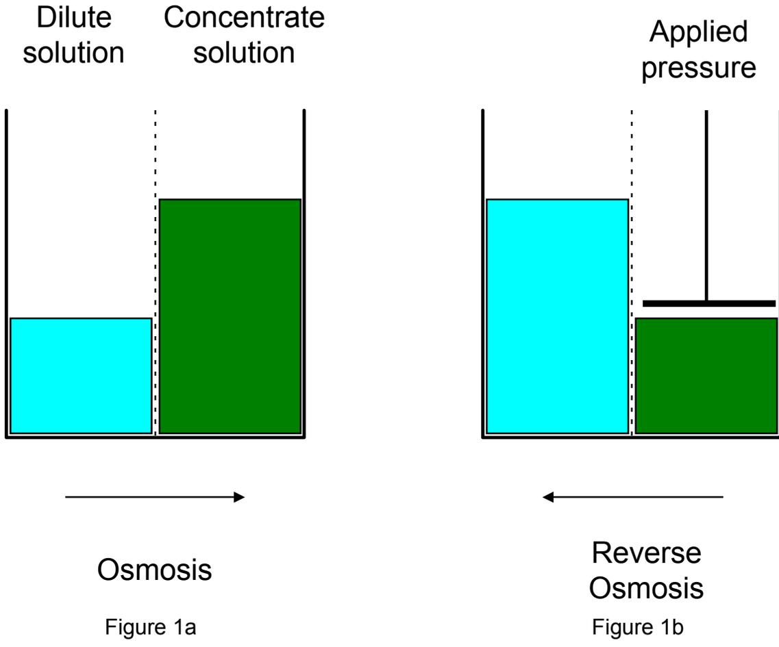
The driving force of the reverse osmosis process is applied pressure. The amount of energy required for osmotic separation is directly related to the salinity of the solution. Thus, more energy is required to produce the same amount of water from solutions with higher concentrations of salt.
