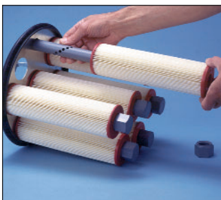
Install cartridge on holding rod.
